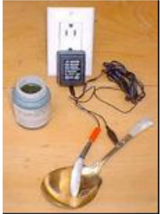
If the plating has black streaks, speed up the wand action and press down harder. A few more passes over the blackened area will clean it up. This is especially prevalent with silver plating. The black streaks will come off with a liquid hand polish after plating.
